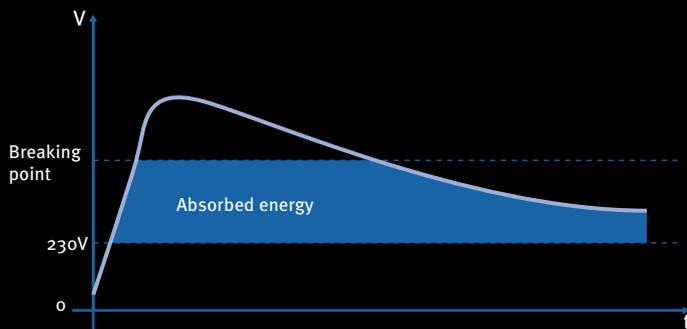
This device functions in common and differential manner at the same time, by absorbing any excessive voltage and discharging it, depending on its nature, towards earth or neutral.
