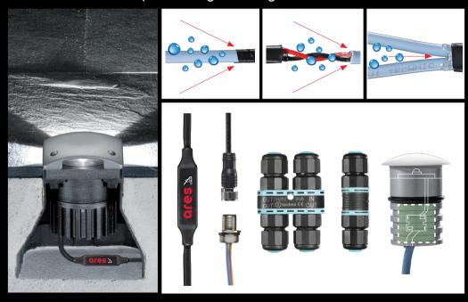
An inaccurate installation of the luminaire with ineffective connection (insulating tape, self-amalgamating tape or sheath inaccurately used) may lead to water passage along the cable and consequently water ingress in the fitting.
